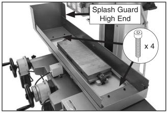
Figure 24. Splash guard base attached.
